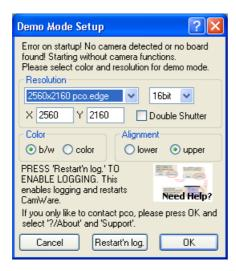
If Camware is started with no camera connected to the PC or with cameras switched off, it starts in demo mode.
