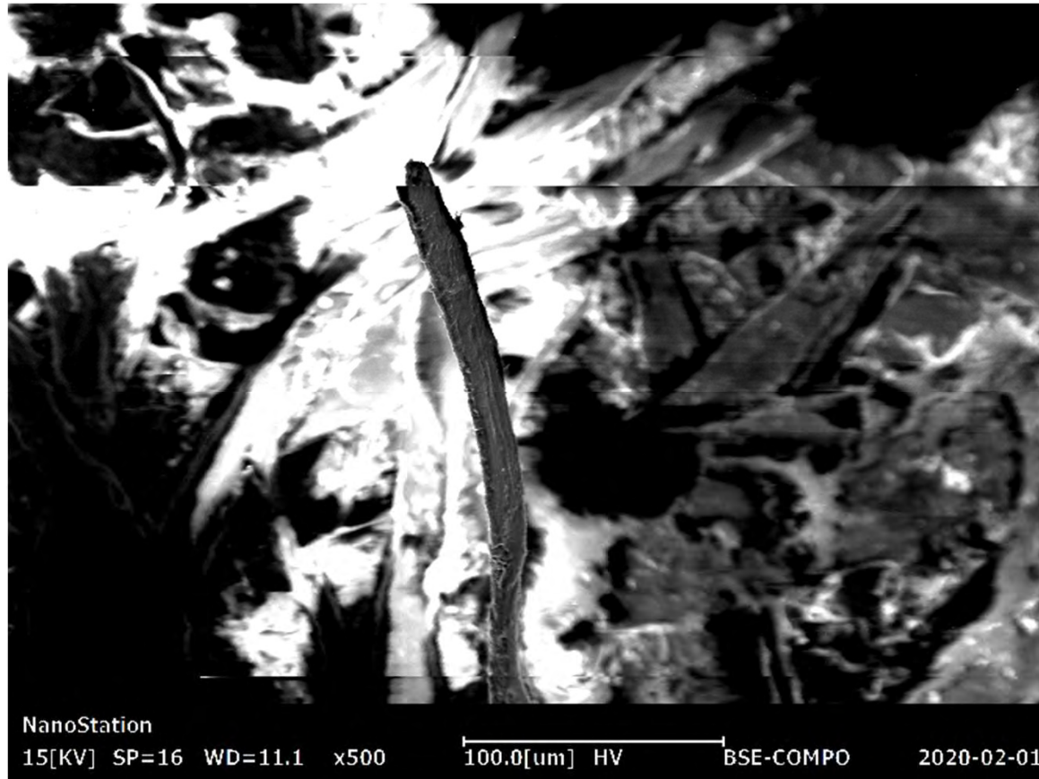
High Vacuum – Chamber at 0.5 Pa (charging prevents imaging)
