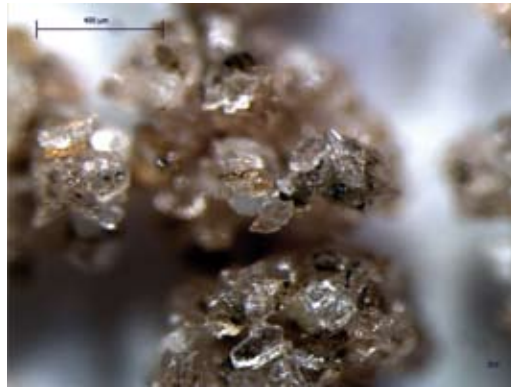
Fig. 5: Aggregated aluminium oxide crystals of abrasive cloth. The crystal dimensions allow different grinding capabilities.
