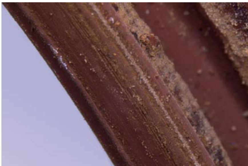
Fig. 1: Bearing seal of a truck: rubber wear after stress test
