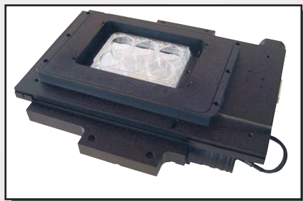
Inset Photo: NanoScanZ Piezo 400 micron stage mounted on a Prior Scientific ProScan™III HI 17 motorized stage.
