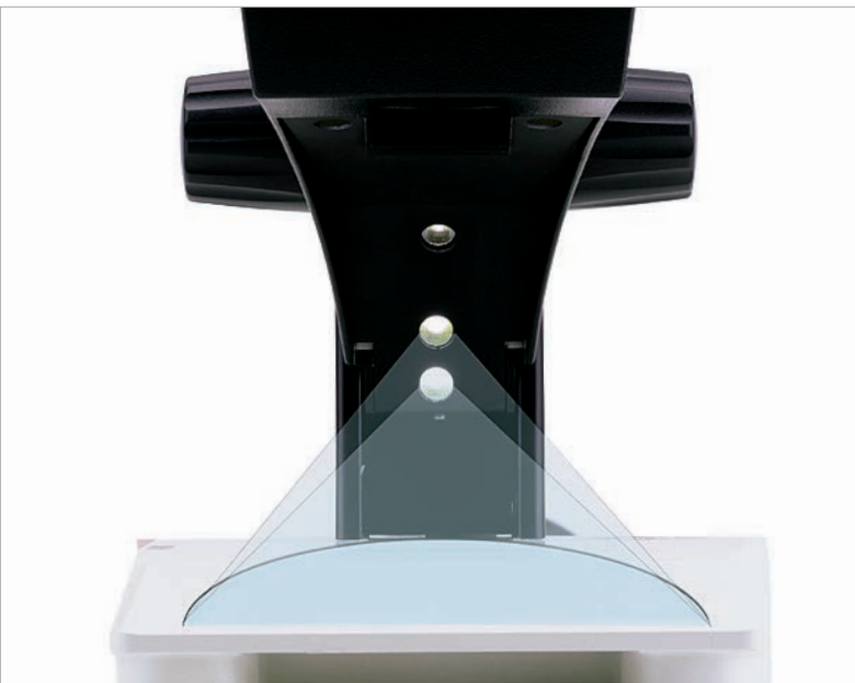
Stage 1 incident light: all five LEDs are lit for maximum intensity.
