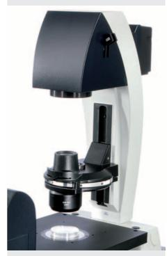
Transmitted light arm with integrated 30 W lamp house and compact S40/0.50 condenser, specifically for micromanipulation.
