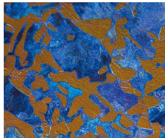
Ferrite C60, hypoeutectoid pearlite, N Plan 50x, DIC
