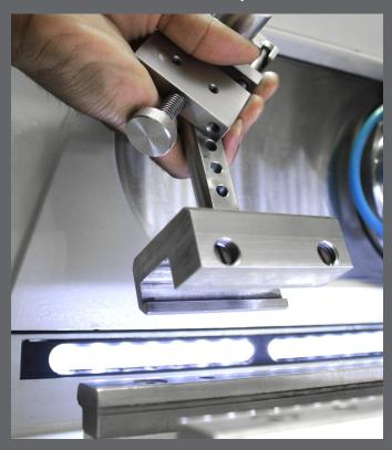
Buehler's Rapid Rail System allows users to secure samples in the cutting chamber and begin the next cut within seconds.
