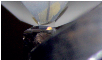
Diamond miller Si sample trimming
