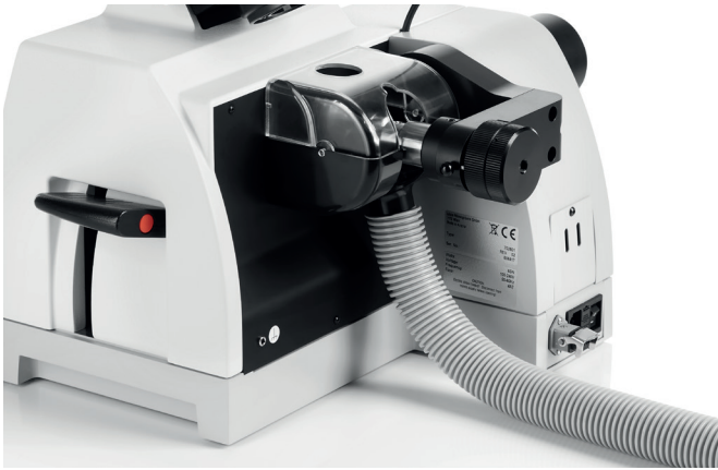
Waste connection to the extraction and filtration unit.
