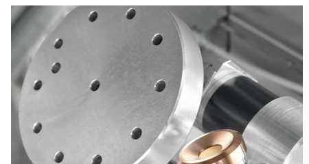
LARS (low angle rotary shadowing) stage for secure mounting of SEM stubs.
