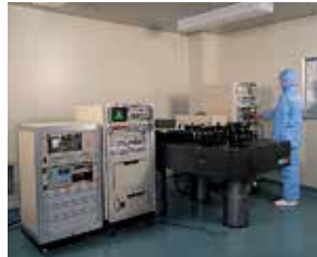
Lodine absorption stabilised He-Ne (633 nm) laser for length measurement
