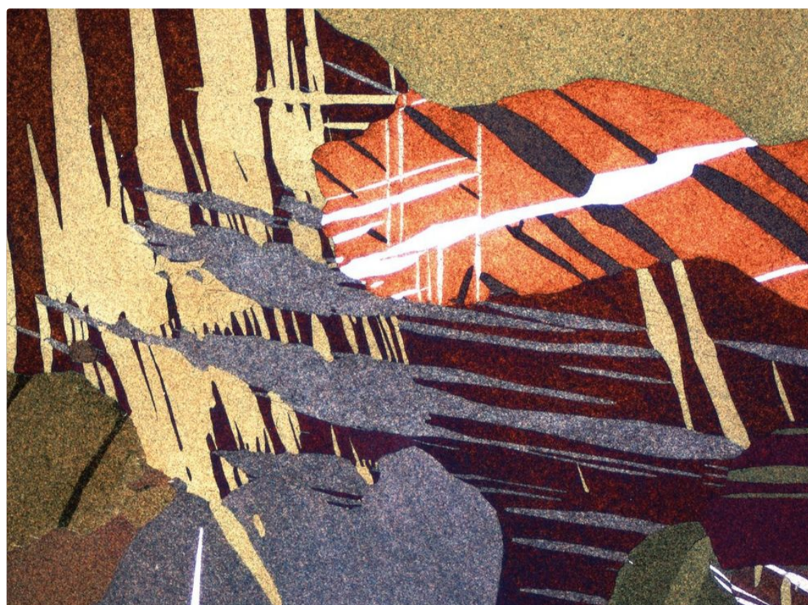
Figs. 16–18 (from left to right): Polarization with and without color etching: Fig. 16: SnPb tin solder, twinning shows deformation at the solder point (K) Fig. 17: Sn dynamically deformed, the pronounced formation of deformation twinning is a sign of a dynamic load (K) Fig. 18: Slip bands due to pronounced deformation on a CuZn wire with fcc lattice (K).
