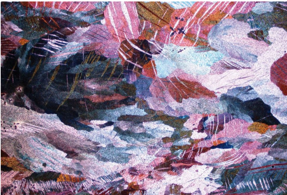
Figs. 13–15 (from left to right): Polarization with and without color etching: Fig. 13: Niobium, cold-formed (B) Fig. 14: Cobalt, cold-rolled (B) Fig. 15: Zinc with twinning due to dynamic deformation (K)
