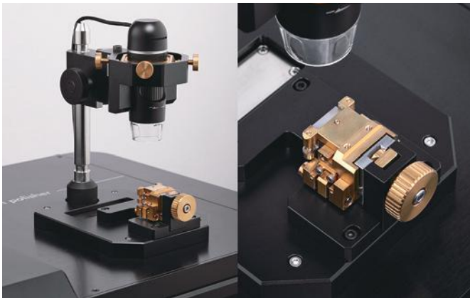
3. Fix the sample stand to the digital microscope.
